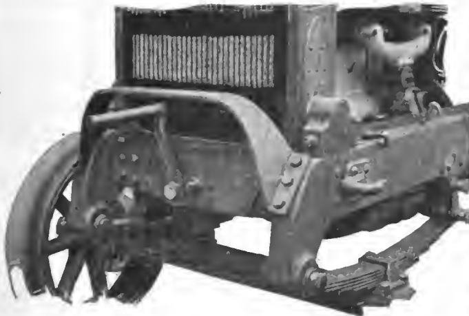
Four views of the Fiat army tractor, showing some of its constructional features. Upper left—Motor of 5.1 by 7.8-in. bore and stroke. Note position of water pump and inlet pipes. Upper right—Rear of chassis. Note cast-steel wheels, which set across frame and spring shackles, forming oil reservoir. Lower left—Radiator is mounted in front with substantial guard. The starting crank is large enough for three men to take hold at once. Note spring assembly. Lower right—The other side of the motor. Note the neat arrangement of the exhaust manifold.
